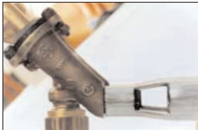
The propane burners installed in our barbecue use fuel-air pre-mixers.
