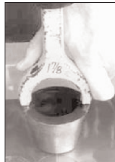
Punching PEM from sheet with arch punch
