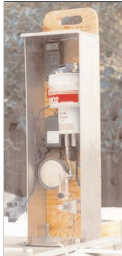
The Panametrics XMO2 oxygen analyzer measures the amount of O 2 in the hydrogen.
