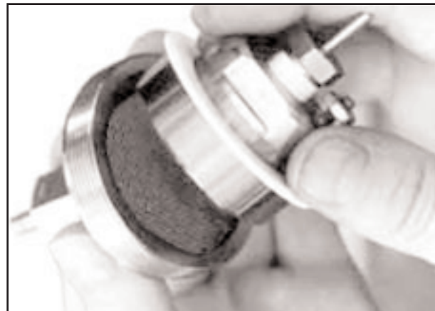
Fuel cell disassembled, showing a gas distribution plate on the left.
